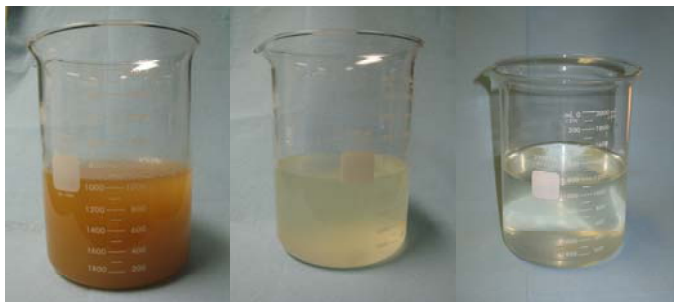
Figure 10. Photographs of fecal simulant and water mixture before and after treatment in the low temperature wet oxidation system.
