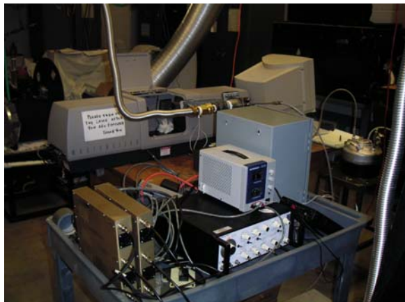
Figure 6. Laboratory wind tunnel setup for droplet size measurements.
