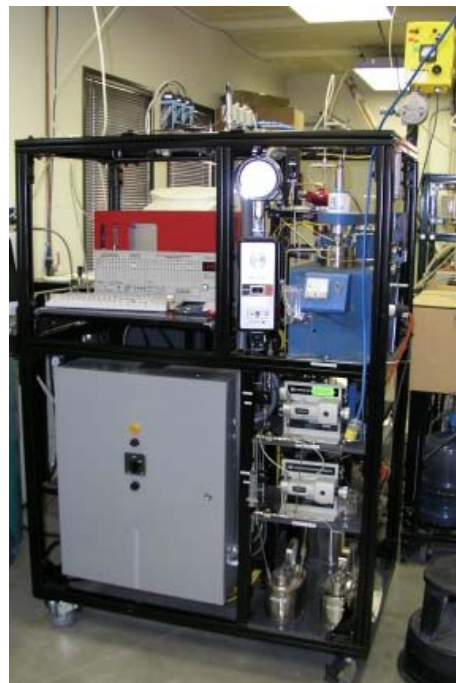
Figure 2. Bench-scale continuous hydroformylation apparatus.
