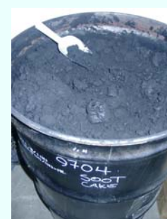
A 55-gallon drum of xylene-extracted combustion soot, still full of giant fullerenes waiting to be recovered!
