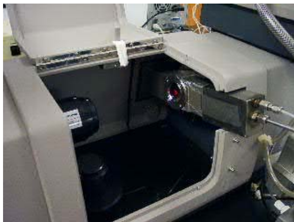
Figure 12. Malvern Mastersizer with nitrogen purged fuel injection fixture.
