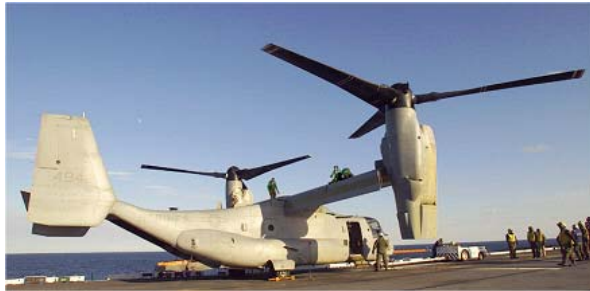
Figure 2. V22 Osprey; Falling is a major safety concerns during exterior maintenance, which requires walking along the wing.
