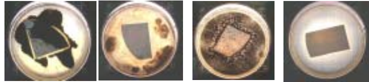
Imbedded Biocide (0.225% IPBC) Zero fungal growth
